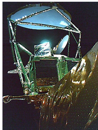
Figure 4. Deployed AMSR2 antenna
