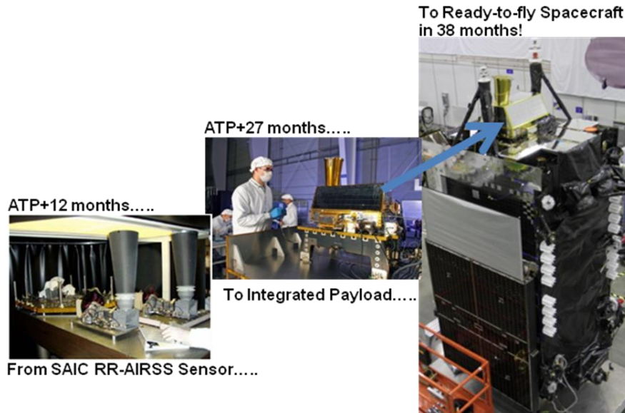
Figure 1. CHIRP launched 39 months from contract authorization to proceed (ATP). A single quadrant of the SAIC RR-AIRSS sensor was integrated to the SES-2 commercial GEO spacecraft delivered 38 months from ATP and launched a month later.
