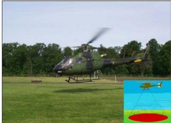
*Figure 19. AGS Monitoring: 1) Left, monitoring helicopter and diagram showing monitoring principle. Normal measuring height is about 100 m. 2) Right, results from AGS monitoring survey of Risø DTU, which is the only site in Denmark that had a nuclear installation.*
