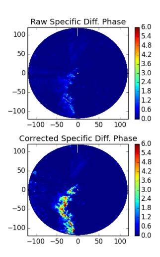
Phase processing performed using a LP based algorithm (Giangrande et al, JTech, 2013)
