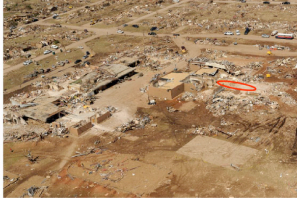
Figure 4-5. Post-tornado aerial view (looking northeast) of the Plaza Towers Elementary School taken May 21, 2013. Much of the debris had already been moved by the time of this photograph as part of the search and rescue operations. The area circled in red shows the approximate location in the hallway of the new main classroom building where the 7 fatalities occurred.
