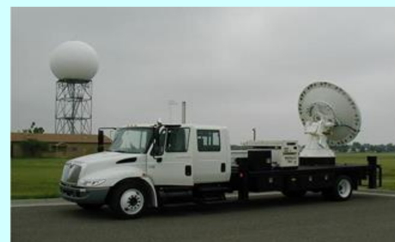
Fig. 1. The data have been collected with three polarimetric S band WSR-88Ds and the mobile X band dual-polarization NOXP.
