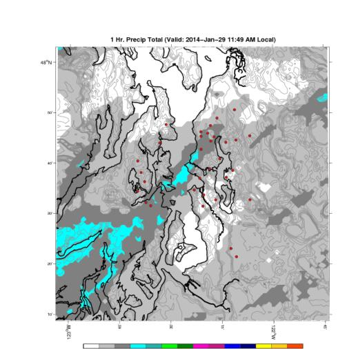
Rainfall estimates derived from radar are calibrated with SPU (and other area) rain gauges.
