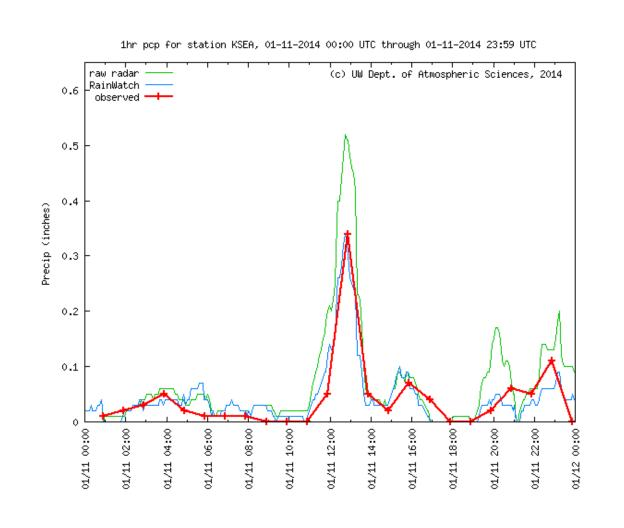
Nowcasts are made using radar echo motion vectors and are extrapolated outward temporally and spatially; accuracy is verified.
