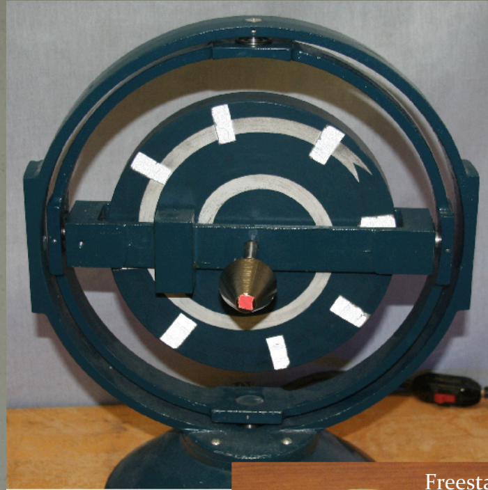
MITAC mechanically driven, gimbal-mounted gyroscope
