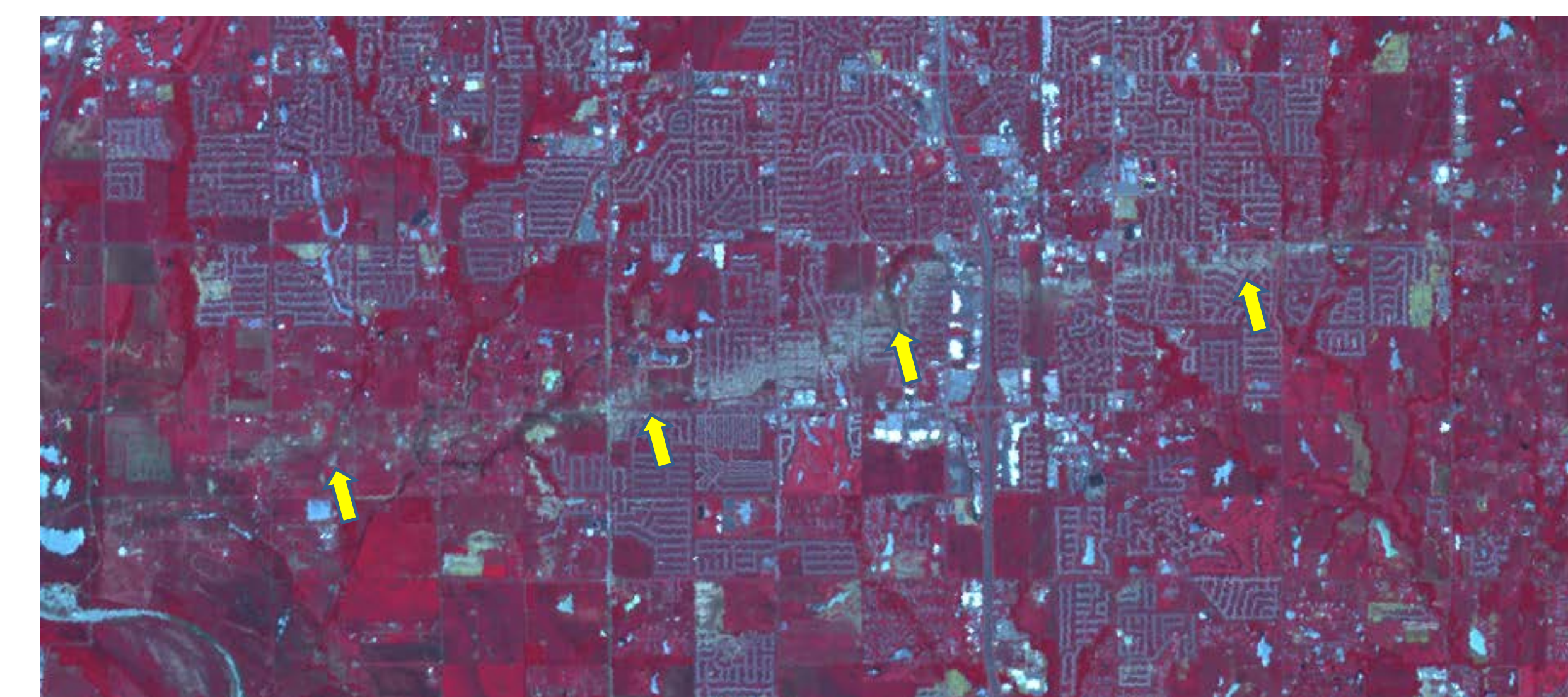
Figure 5: An ASTER false color composite from 2 June 2013 shows where vegetation and urban infrastructure have been disturbed in Moore, OK. Changes in tornado path and width can also be seen.
