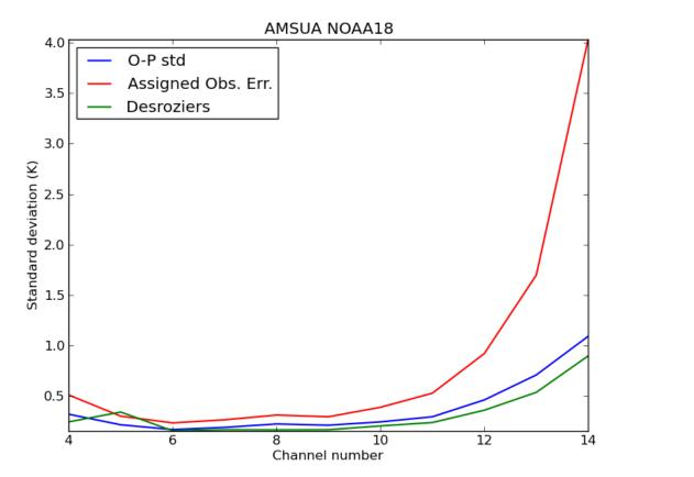
Large assigned errors for ch 13-14 To avoid temperature drift near model top
