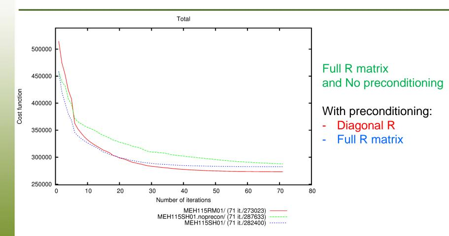
Full matrix: Desroziers error correlation is used, retaining operational errors on diagonal
