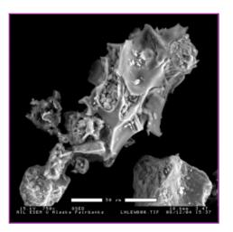
Ash collected from the leading edge of the wing of a commercial aircraft that had a nondamaging encounter with the Kasatochi volcanic cloud.
