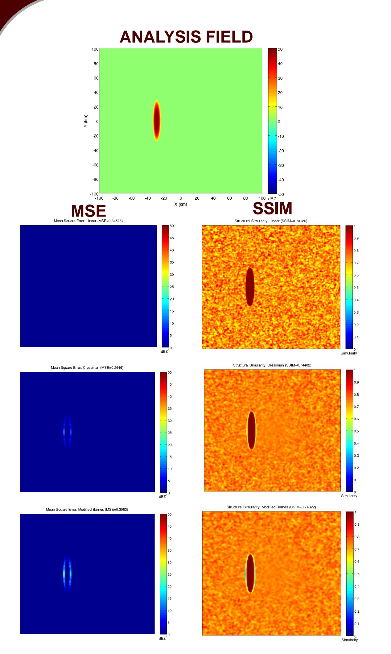
The first analysis field depicts a simulated storm cell or linear system centered about 20-40km west of the radar. The second analysis field depicts a "checkerboard" domain with concentric cells of negative and positive data. The analysis fields were sampled onto a polar grid and interpolated onto Cartesian grid with each different scheme. Input data had additive Gaussian noise with a mean of 0 and variance of 50.
