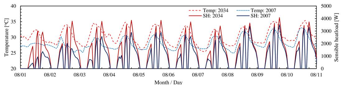
Time series of outdoor air temperature and sensible heat (SH) load in the LDK in 2007 and 2034
