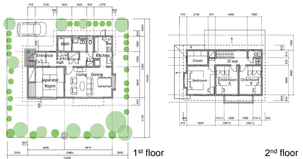
Plans for a model house used for BES (a standard detached house in Japan)
