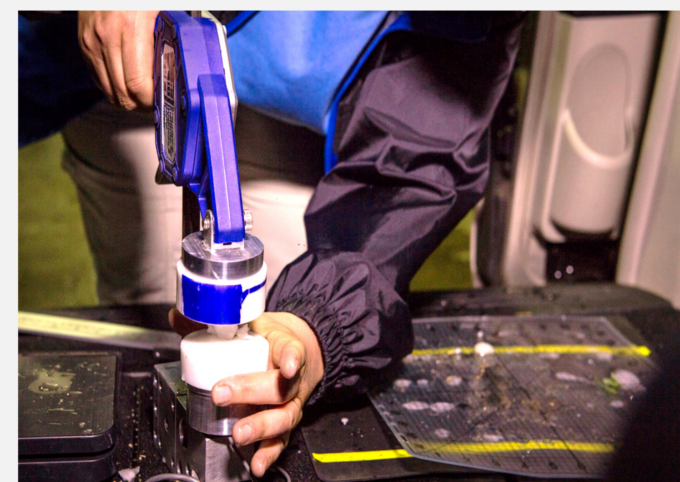
Figure 3. Compressive force test being conducted on a hailstone on 18 May 2013.
