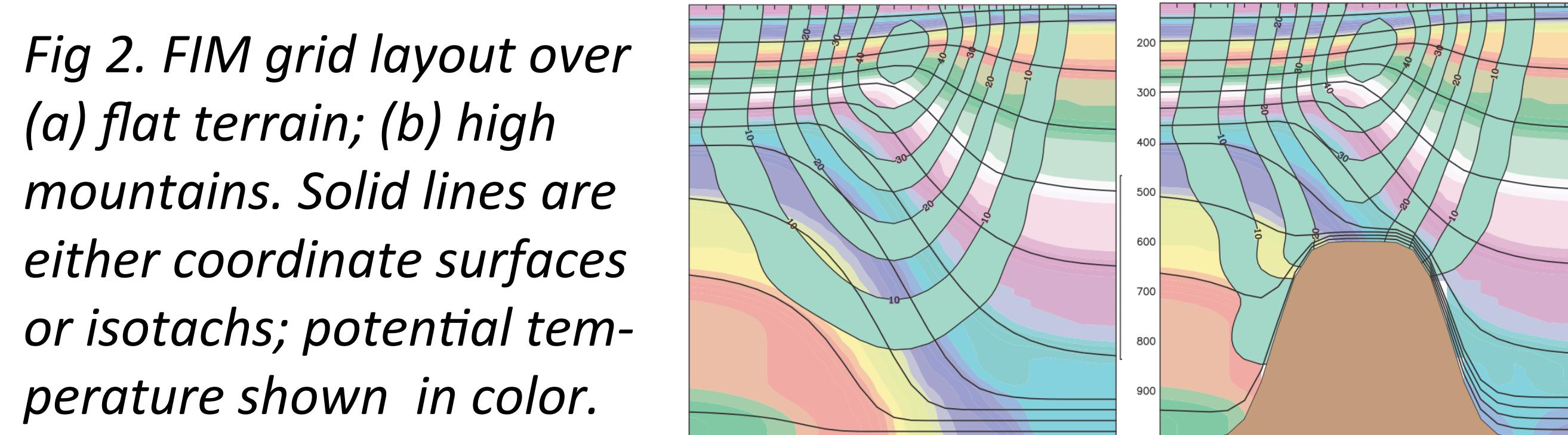
Fig 2. FIM grid layout over (a) flat terrain; (b) high mountains. Solid lines are either coordinate surfaces or isotachs; potential temperature shown in color.
