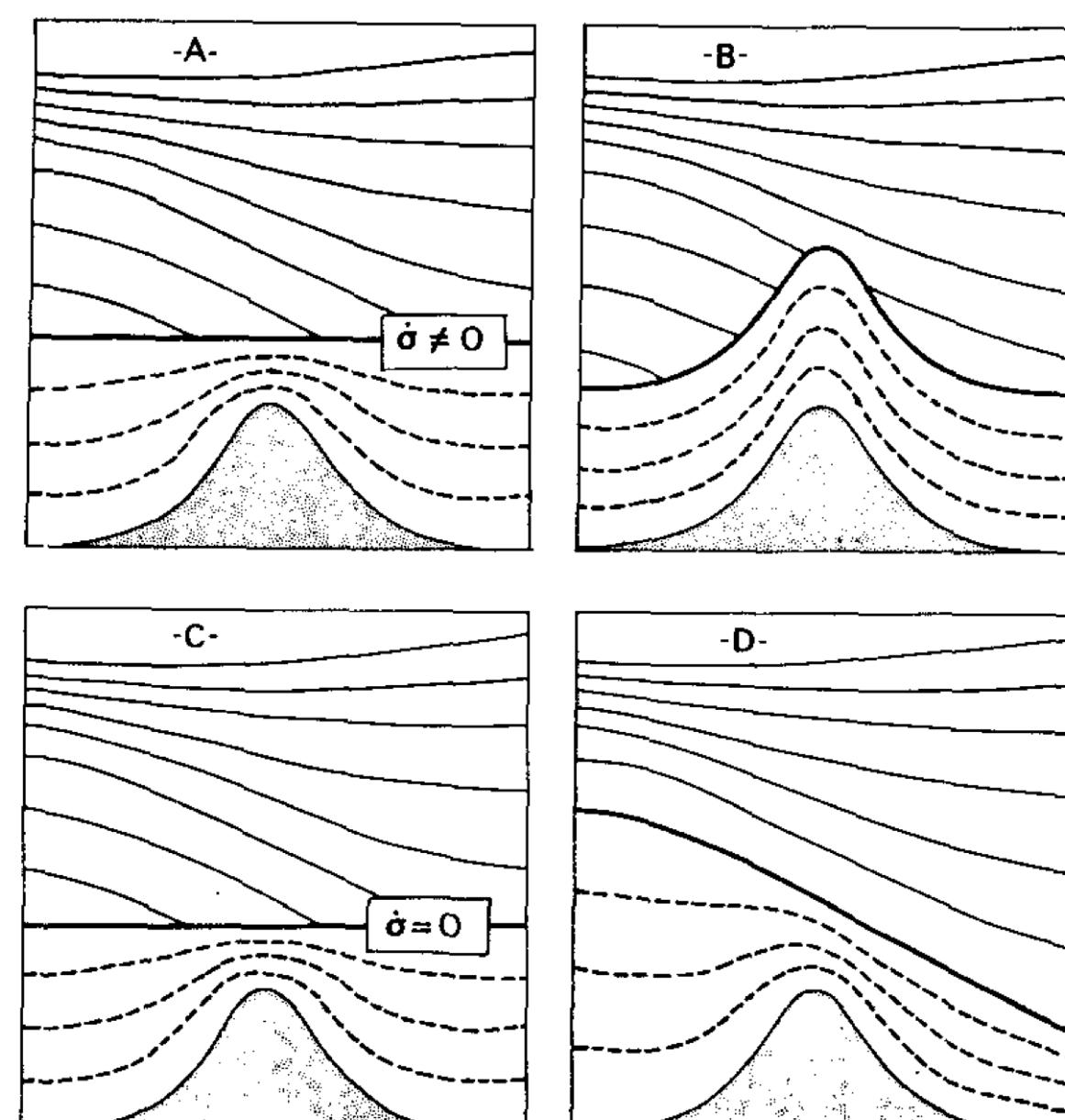
Fig 1. Four ways to avoid coordinate-ground intersections (from Bleck, 1978). Coordinate layers below the heavily drawn interface are to various degrees non-isentropic. The interface is fixed (i.e. permeable) in schemes A,B; material (i.e. flow-following) in schemes C,D.
