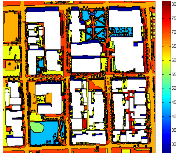
Figure 9: Contours of T_{mrt} (°C) at 1200 LST in Future August. The buildings are indicated in white.
