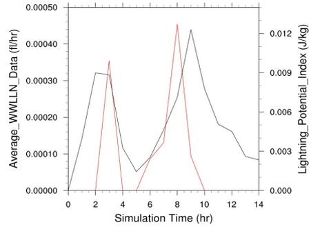
Figure 7: WWLLN (red) and LPI (black) calculated with the Thompson et al. 2004 microphysical parameterization.
