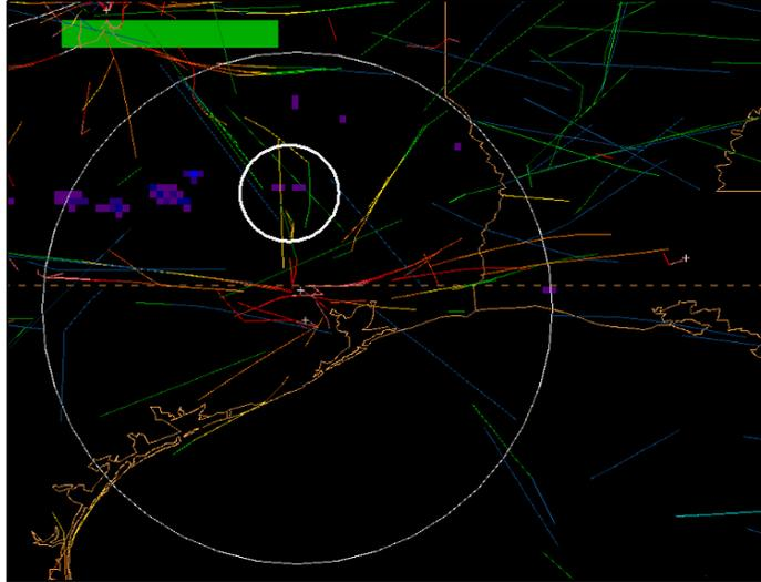
**Figure 9.** A pseudo-geostationary lightning mapper flash extent density mosaic display in N-AWIPS from the Houston lightning mapping array at 2002 UTC on 15 August 2013 during the Aviation Weather Center's Summer Experiment. The large circle is the rough range of the network. The small circle is the region of interest. The various colored lines are the flight tracks of aircraft.
