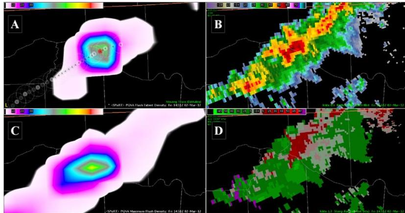
**Figure 2.** An AWIPS II four panel display demonstrating the pseudo-geostationary lightning mapper (PGLM) flash extent density (A), radar reflectivity (B), PGLM 30 min maximum flash density (C), and storm relative velocity (D). The dots and circles in panel A are part of the Total Lightning Tracking Tool shown in Fig. 4.
