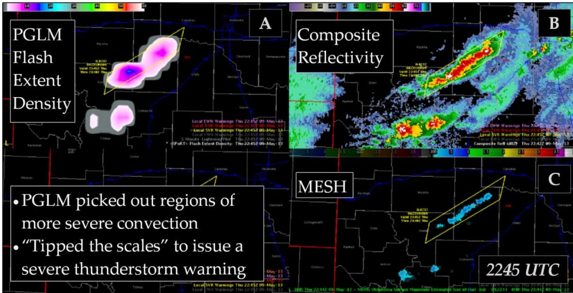
**Figure 8.** An AWIPS II four panel display showing the pseudo-geostationary lightning mapper flash extent density (A), composite radar reflectivity (B) and radar derived maximum estimated size of hail (C) at 2245 UTC in Central Oklahoma at 9 May 2013.
