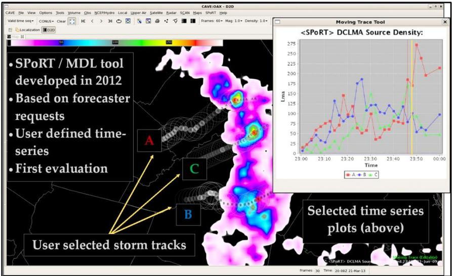
**Figure 4.** An example of how the total lightning data are viewed in AWIPS II (example from the Washington D.C. domain) with the cell tracks plotted for three cells in the main display. The pop-up window in the upper right shows the actual time series display for all three selected cells. The vertical yellow bar in the pop-up display corresponds to the current time in the AWIPS II display.
