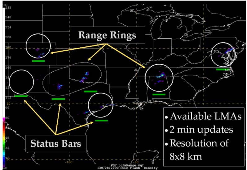
**Figure 3.** An example image of the pseudo-geostationary lightning mapper (PGLM) PGLM mosaic product as it would appear in N-AWIPS for NASA SPoRT's national center end users. The rings indicate the approximate range of the best observations from each ground-based lightning mapping array. The horizontal bars represent the status of each individual network. In this case, all of the bars are green indicating there are no issues with any network.
