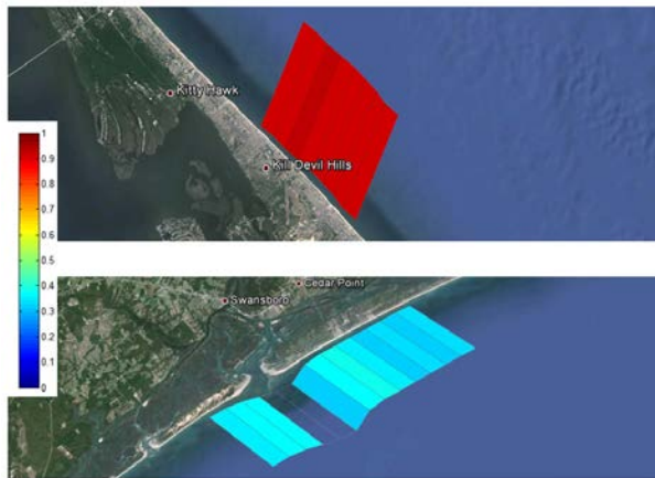
Figure 11. An example of the rip current forecast model output shown spatially on a map for both KDH (top) and EMI (bottom).
