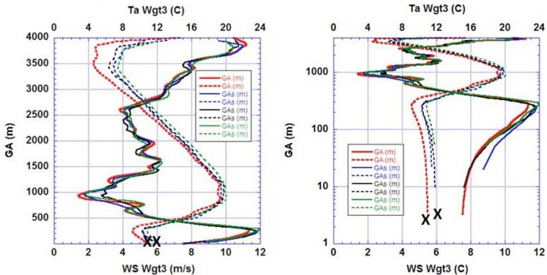
**Figure 5.** Comparison from CIRPAS Twin Otter aircraft between YES XDD and Vaisala RD94 dropsonde observations of wind speed (solid), WS and air temperature (dashed), Ta – Flight 2, 25 June 2011: linear geopotential height coordinates on the left, log coordinates, emphasizing boundary layer detail, on the right. Vaisala data is in red, YES data in Blue, black and green. X is data from NDBC buoy 46042.
