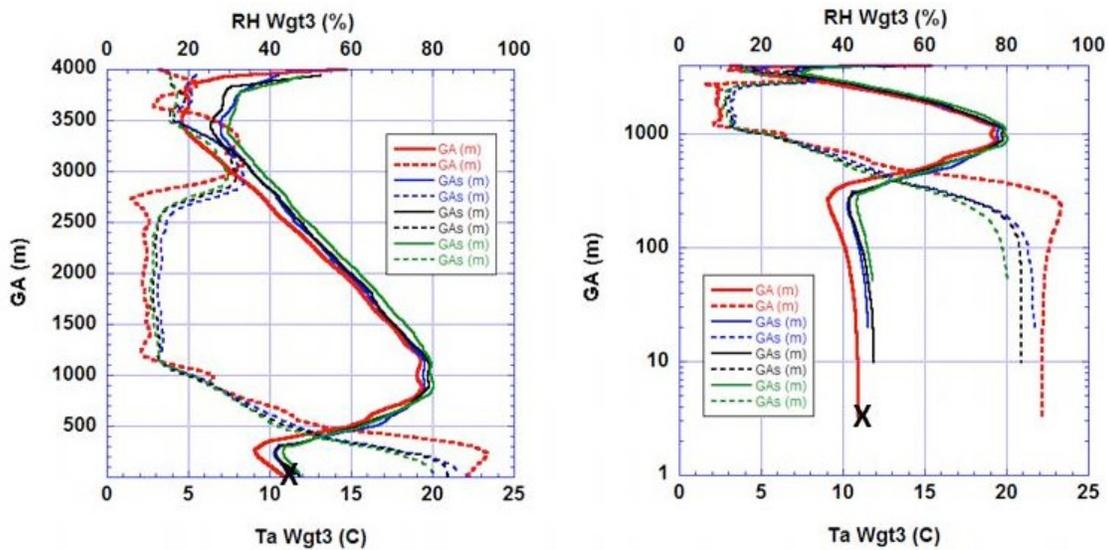
**Figure 4.** Comparison between YES XDD and Vaisala RD94 dropsonde observations from CIRPAS Twin Otter aircraft of Ta, air temperature (solid) and RH, relative humidity (dashed) during Flight 2, 25 June 2011 vs a) linear geopotential height (left) and b) log geopotential height (right), designed to emphasize boundary layer detail. RD-94 data is in red, XDD data in blue, black and green. X is data from NDBC buoy 46026.
