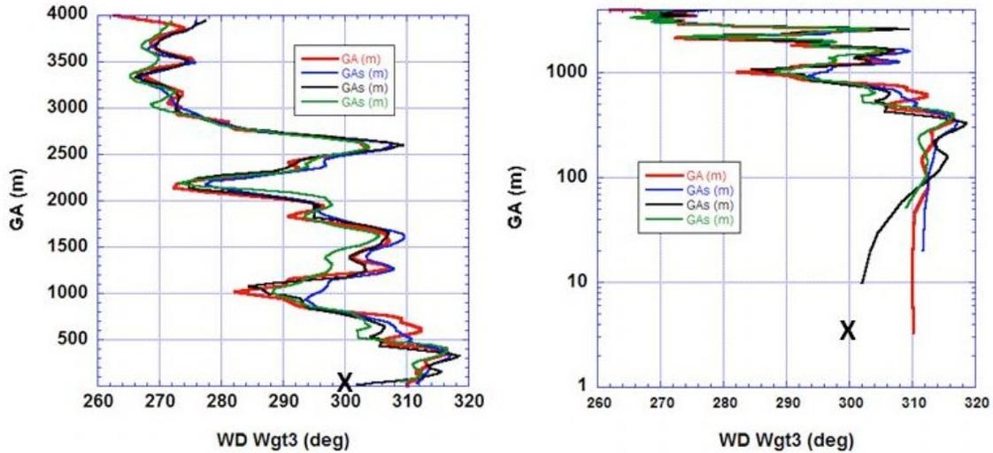
**Figure 6.** Comparison from CIRPAS Twin Otter aircraft between YES XDD and Vaisala RD94 dropsonde observations of wind direction WD– Flight 2, 25 June 2011: linear geopotential height coordinates on the left, log coordinates, emphasizing boundary layer detail, on the right. Vaisala data is in red, YES data in blue, black and green. X is data from NDBC buoy 46026.
