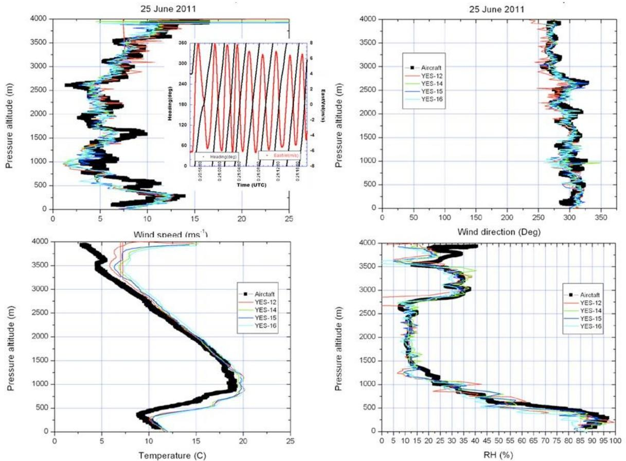
**Figure 7.** Comparison of XDD sonde profiles with Twin Otter aircraft vertical profiles during spiral descent on 25 June over buoy 46026 of a) wind speed (upper left), b) pressure (upper right), c) temperature (lower left) and d) relative humidity (lower right). Inset shows the the aircraft heading and east-west component of the wind as a function of time.
