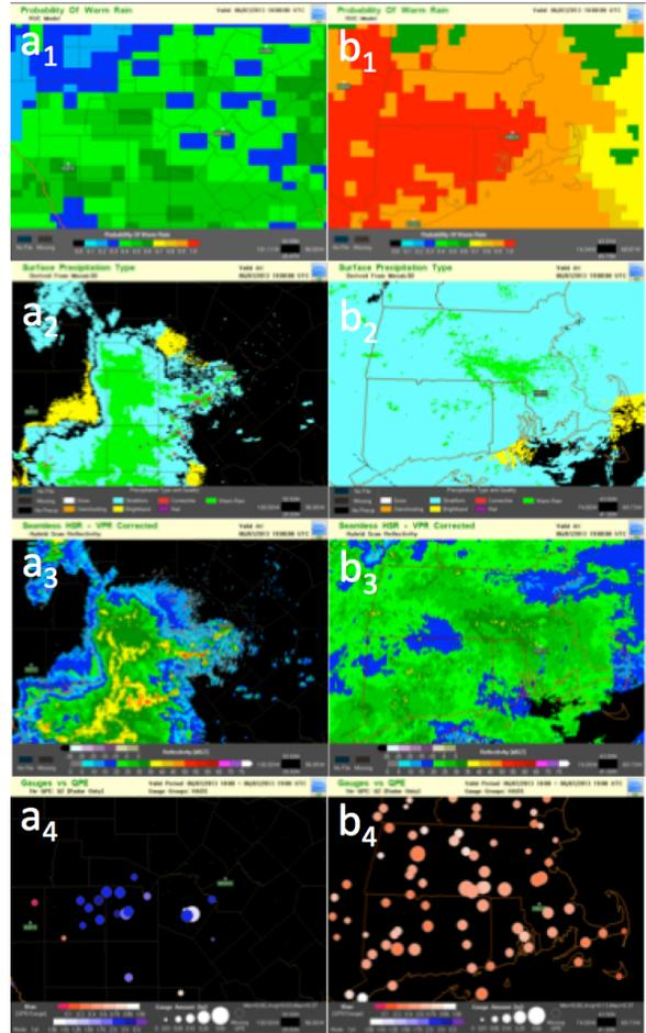
Figure 9 The POWR fields valid at 19:00UTC on 9 June 2013 in south Texas (a<sub>1</sub>) and northeastern US (b<sub>1</sub>), Corresponding NMQ surface precipitation type (a<sub>2</sub> and b<sub>2</sub>), SHSR (a<sub>3</sub> and b<sub>3</sub>), and bias ratio maps of the hourly NMQ radar QPE vs. gauges (a<sub>4</sub> and b<sub>4</sub>) are also shown.
