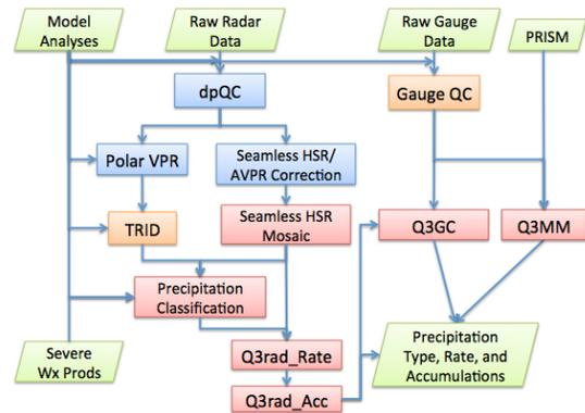
Figure 2 MRMS QPE process data flow. The green parallelograms at the top show the input data from different sources, and those at the bottom show the MRMS product outputs. Note that the MRMS severe weather products are inputs for the precipitation classification. Blue boxes indicate processes applied to single radar volume scan data, pink boxes represent processes applied on the MRMS CONUS Cartesian grid, and orange boxes indicates point data or profile data processes.
