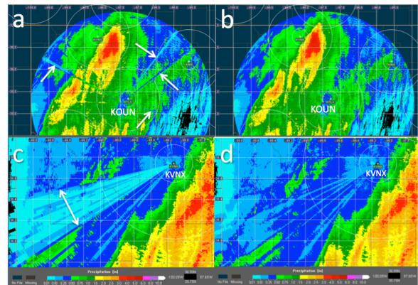
Figure 5 Example QPE accumulation fields without the non-standard blockage mitigation (a, c) and with the mitigation (b, d). White arrows indicate areas of discontinuities due to cellphone and water towers (a) and growing trees (c).
