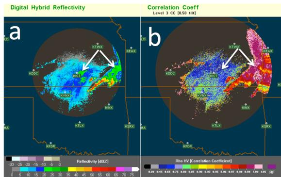
Figure 3 Base reflectivity (a) and correlation coefficient (b) fields from KICT radar valid at 06:00UTC on 20 May 2013. The two white arrows indicate areas of anomalous propagation and biological echoes towards the west and an area of precipitation to the east.
