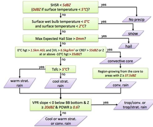
Figure 8 The surface precipitation classification process in the MRMS system.
