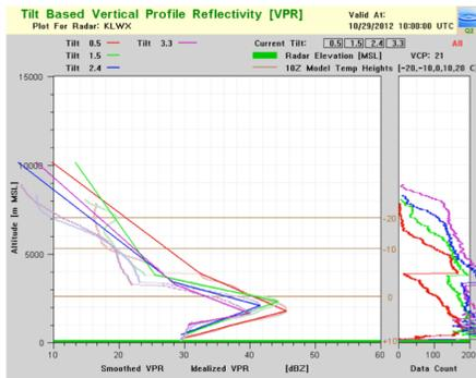
Figure 6 AVPRs from KLWX radar at 10:00UTC on 29 Oct. 2012. Colored curves in the main panel show profiles of azimuthally averaged reflectivities from stratiform precipitation areas on different tilts. The straight lines are the linear fitting AVPRs. Curves in the right panel shows number of data samples associated with the azimuthal mean reflectivities.
