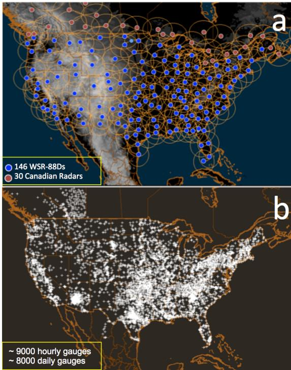
Figure 1. MRMS domain and locations of the radar and rain gauge sites. The blue dots indicate the US WSR-88D radar sites and maroon dots the Canadian radar sites (a). Brown circles are the 250km range rings (a) and white “+”s indicate locations of the hourly and daily gauges (b).
