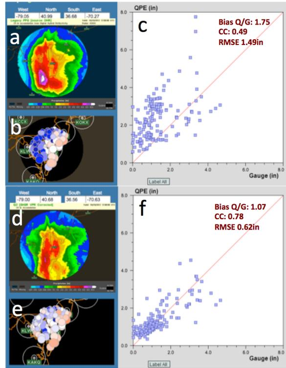
Figure 7 Daily QPE maps before (a) and after (c) the AVPR correction. Bias ratios of the QPEs vs. gauge observations are shown as the bubble charts in panels (b) and (e), respectively. The size of the bubbles represents the gauge amounts and the color represents the QPE bias (pink means underestimation and blue means overestimation). The scatter plots of the two QPEs vs. gauge data are shown in panels (c), and (f), respectively.
