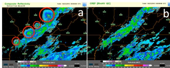
Figure 4 Composite reflectivity fields (a) from the NMQ single-polarization radar QC and (b) from the MRMS dpQC.
