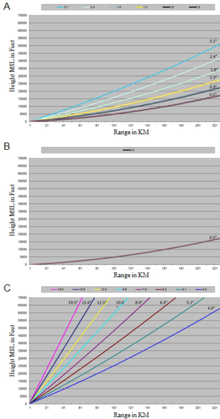
Figure 4: An illustration of a volume scan in which a SAILS cut is inserted into the middle of VCP 12. The radar scans up through the middle of the volume scan to 3.1° (A), transitions down to collect the additional 0.5° split cut (B), then elevates to 4.0° to resume collecting data to complete the volume scan.
