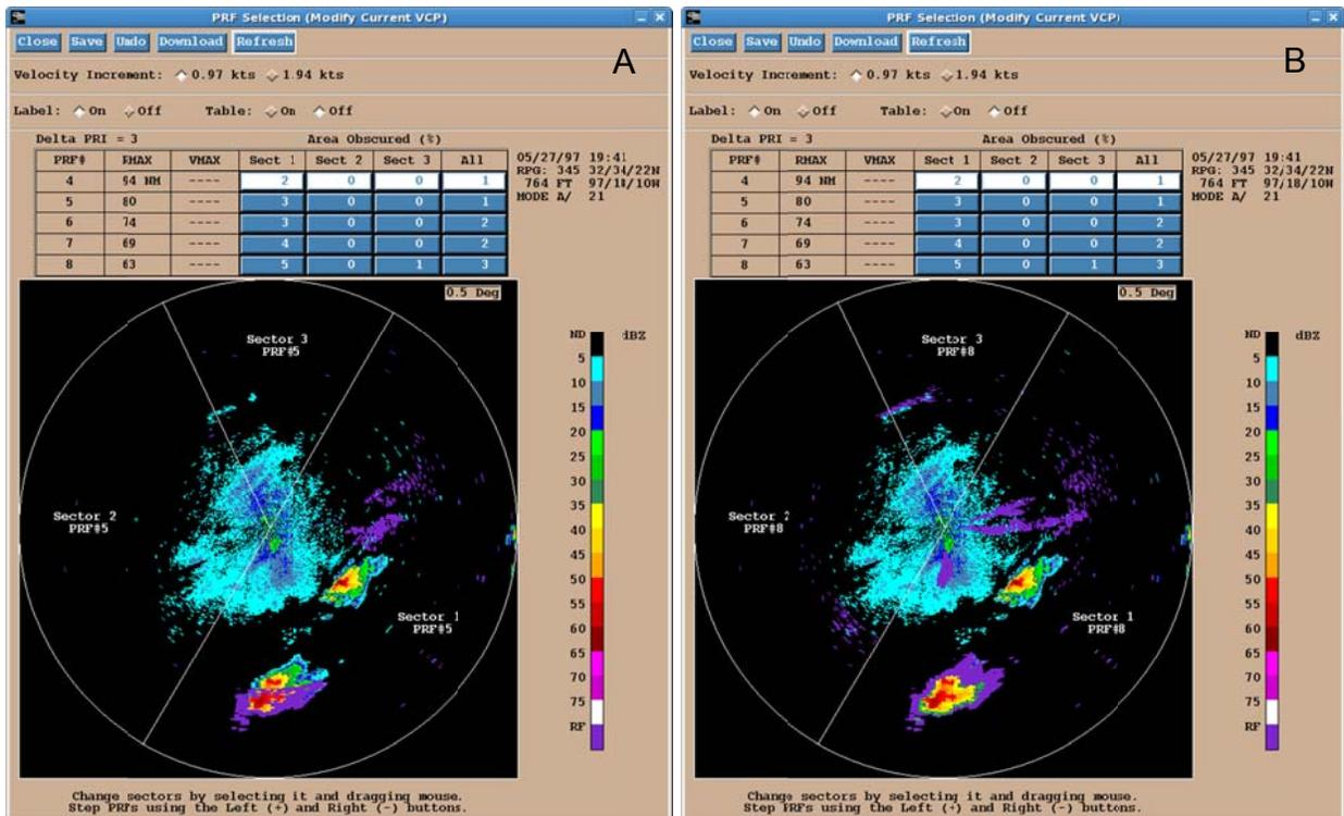
Figure 5: A comparison of the expected range obscured bins using PRF 5 as selected by the baseline Auto PRF algorithm (A) versus the expected range obscured bins using PRF 8 as selected by Storm-Based Auto PRF (B).
