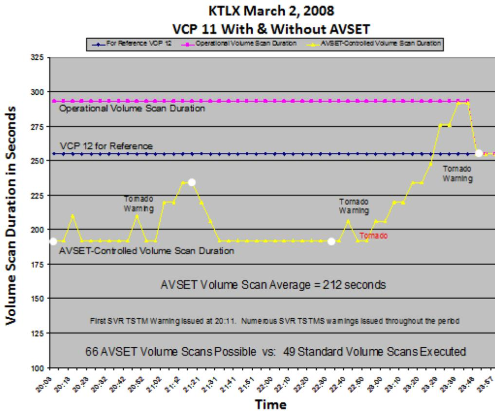
Figure 1: Four reflectivity panels for 02 March 2008 at 20:03 (A), 21:16 (B), 22:30 (C), and 23:48 (D) UTC. The time series chart depicts the duration of the operational volume scan (magenta) versus the AVSET-controlled volume scan (yellow). The four white dots along the AVSET-controlled volume scan correspond to the time of the four reflectivity images. The volume scan duration of VCP 12 (blue) is shown for comparison.
