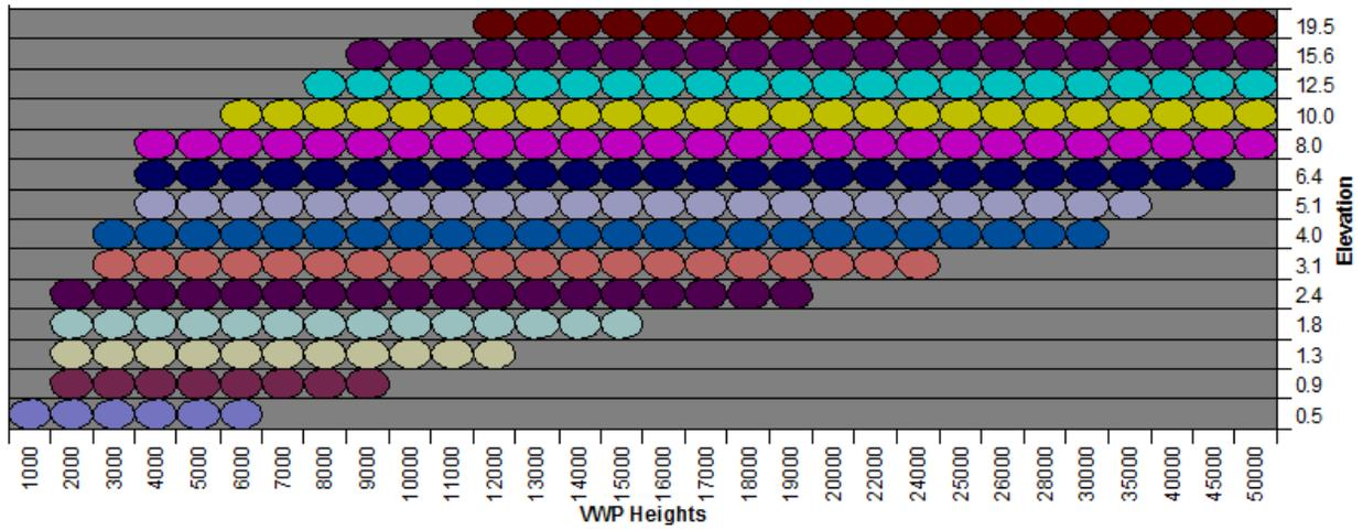
Figure 2: The possible VAD estimates from each elevation angle when restricting the valid slant range to  $\geq 10$  km and  $\leq 120$  km.
