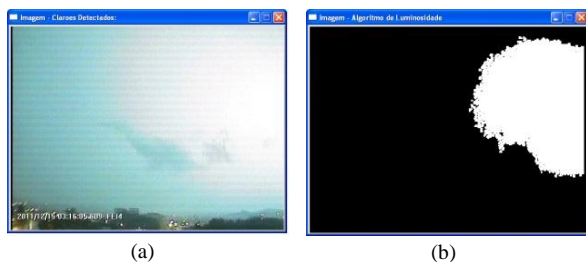
Figure 7: (a): Normal image containing one lightning flash and (b): Dilated Brightness algorithm.
