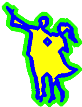
Figure 2: A shape (in blue) and its morphological dilation (in green) and erosion (in yellow) (From Wikipedia, 2013).
