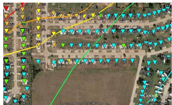
Figure 12: Google Earth image showing several EF0 or EF1 rated duplexes which were subsequently demolished due to debris impacts.
