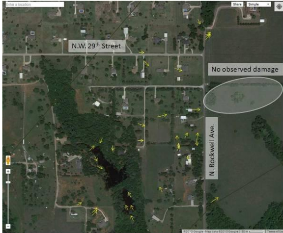
Figure 3: Debris trajectory analysis near N. Rockwell Ave. and N.W. 28th Street in Newcastle. The closest co-located WSR-88D radar volume scan is from KCRI around 1954 UTC.
