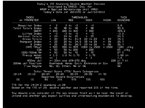
Figure 18. Detailed TTS window displayed in MIDDs provides the user with index and parameter severe thresholds and the specific values derived from the current sounding used to generate the TTS.
