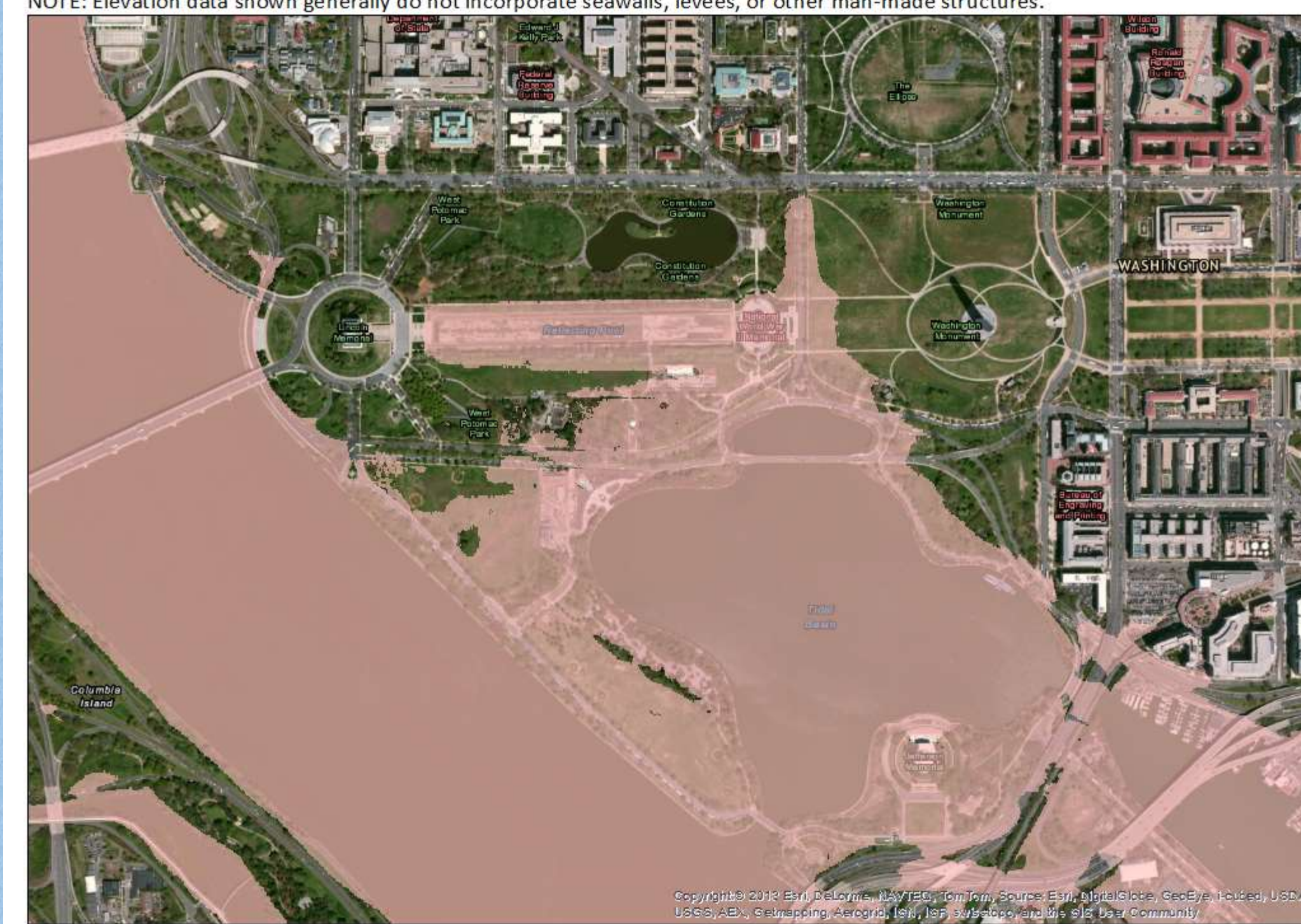
11.6 ft NAVD88 Inundation Area. Elevations are in feet NAVD88. Data shown is 1/9 arc-second. NOTE: Elevation data shown generally do not incorporate seawalls, levees, or other man-made structures.
