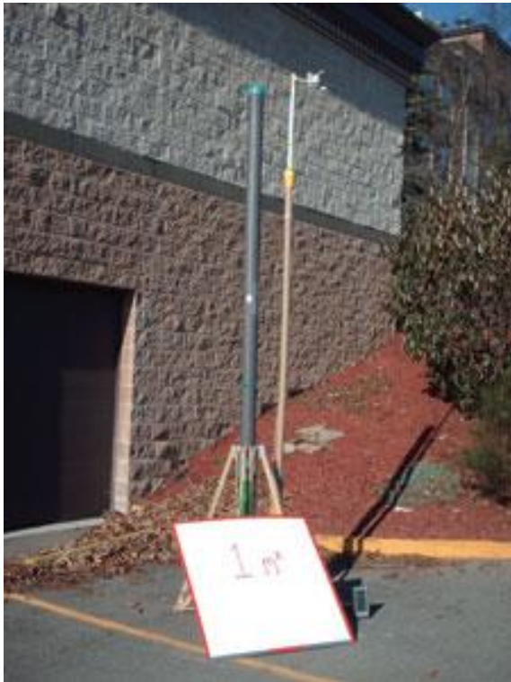
Figure 3: The SuperStack with optional wind sensor near stack top and square-meter board.
