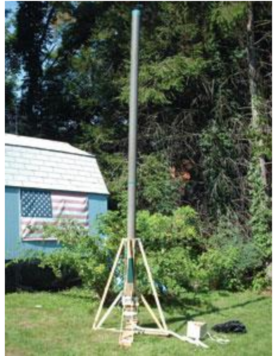
Figure 2: The SuperStack (~ 13 feet tall, 4 inches inside diameter).
