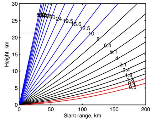
Figure 3: Proposed scan strategy for MPAR: i) long and short uniform PRTs at low elevations (< 1 degree), ii) staggered PRT Beam-Multiplexing (SBMX) for middle elevations (1 ~ 8 degrees); iii) a broad beam at high elevations (> 10 degrees).
