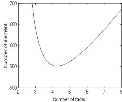
Figure 1: Number of columns/elements as a function of the number of faces. The four-face configuration minimizes the number of elements and is optimal for one beam per face.
