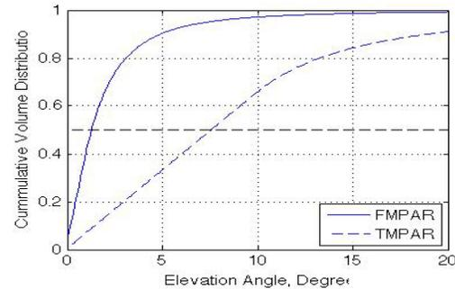
Figure 2: Cumulative volume coverage distribution as a function of elevation.
