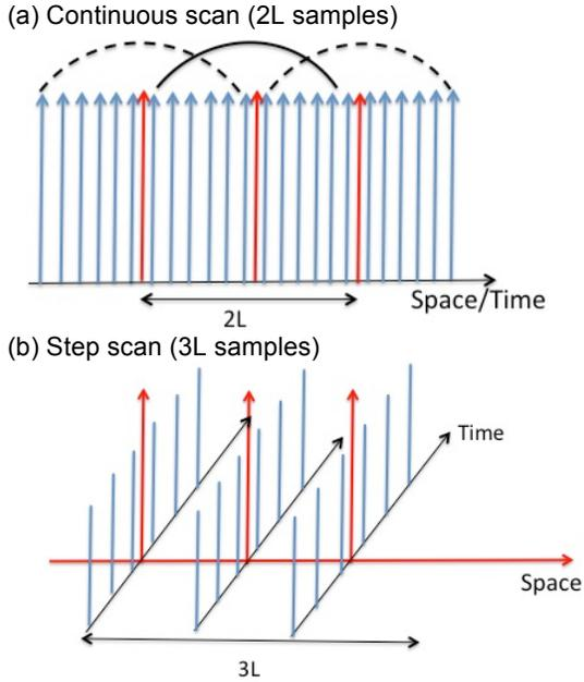
Figure 4: Conceptual sketch of sampling principle for continuous scan (a) with 2L samples for a beamwidth versus that for a step scan (b) which allows 3L samples.
