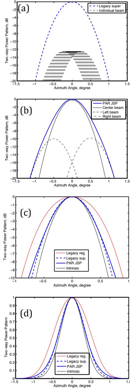
Figure 5: Comparison of antenna patterns between legacy super-resolution beam and the PAR JSP beam: a) legacy super-resolution continuous scan beam patterns, b) PAR JSP step scan beam patterns, and c) & d) comparison of effective beam patterns in decibel and linear unit, respectively.
