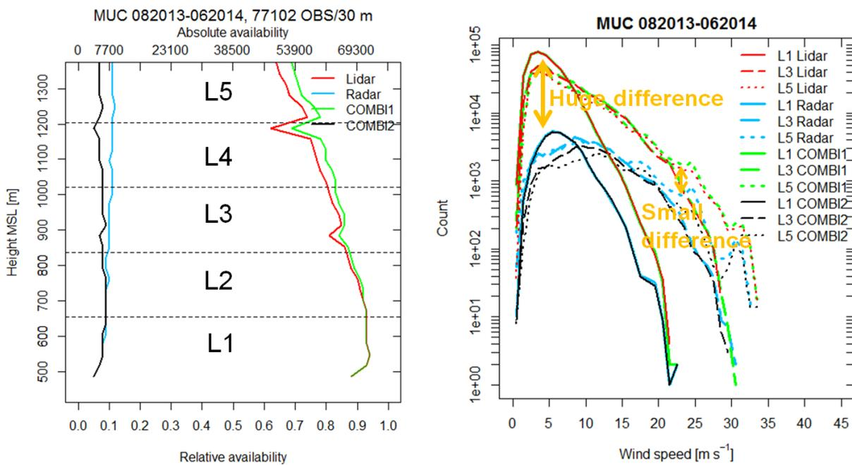
Figure 3: Availability of VVP data from August 2013 until June 2014 at Munich Airport; as a function of layer height (left) and as a function of wind speed (right). COMBI2 represents cases where both sensors provide valid data and COMBI1 where at least one sensor provides valid data.
