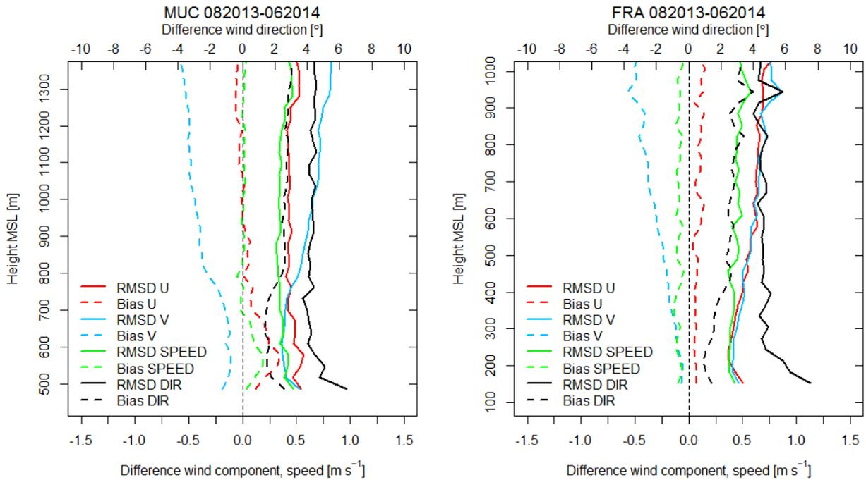
**Figure 8:** Mean lidar-radar RMSD and bias of VVP U and V wind components, wind speed (SPEED) and direction (DIR) from August 2013 until June 2014 for MUC (left) and FRA (right); as a function of height.
