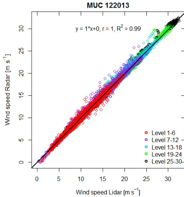
**Figure 7:** Scattergram of lidar and radar wind speed for December 2013 at MUC.
