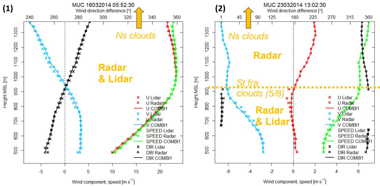
Figure 5: VVP vertical profiles of U and V wind components, wind speed (SPEED) and direction (DIR) of lidar, radar and the combination of both sensors (COMBI1) at MUC. Dates: (1) 16 March 2014, 5.52 UTC; (2) 23 March 2014, 13.02 UTC.
