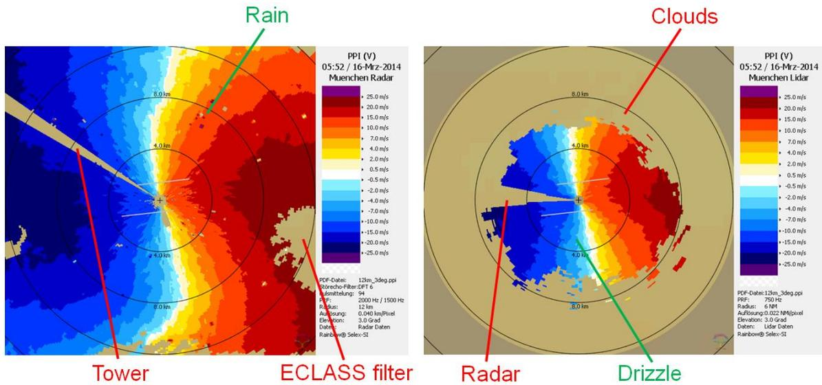
Figure 2: Radar (left) and lidar (right) 3° PPI radial velocity.
