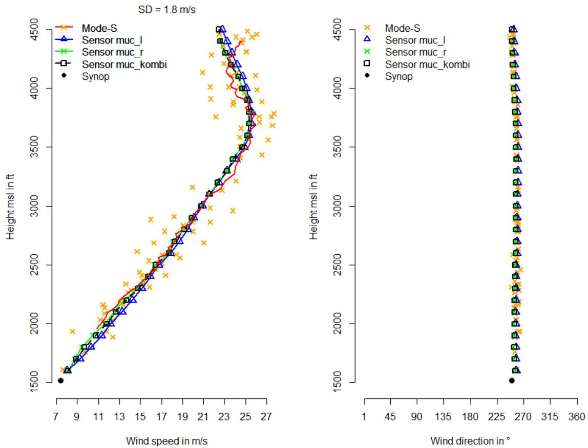
**Figure 9:** Vertical profiles of wind speed (left) and direction (right) of lidar (muc\_l), radar (muc\_r), the combination of both sensors (muc\_kombi) and of Mode-S EHS (Mode-S) at MUC. Date: 04 November 2013, 20:23 UTC till 20:28 UTC for LLWAS wind and 20:18 UTC till 20:33 UTC for Mode-S EHS wind.
