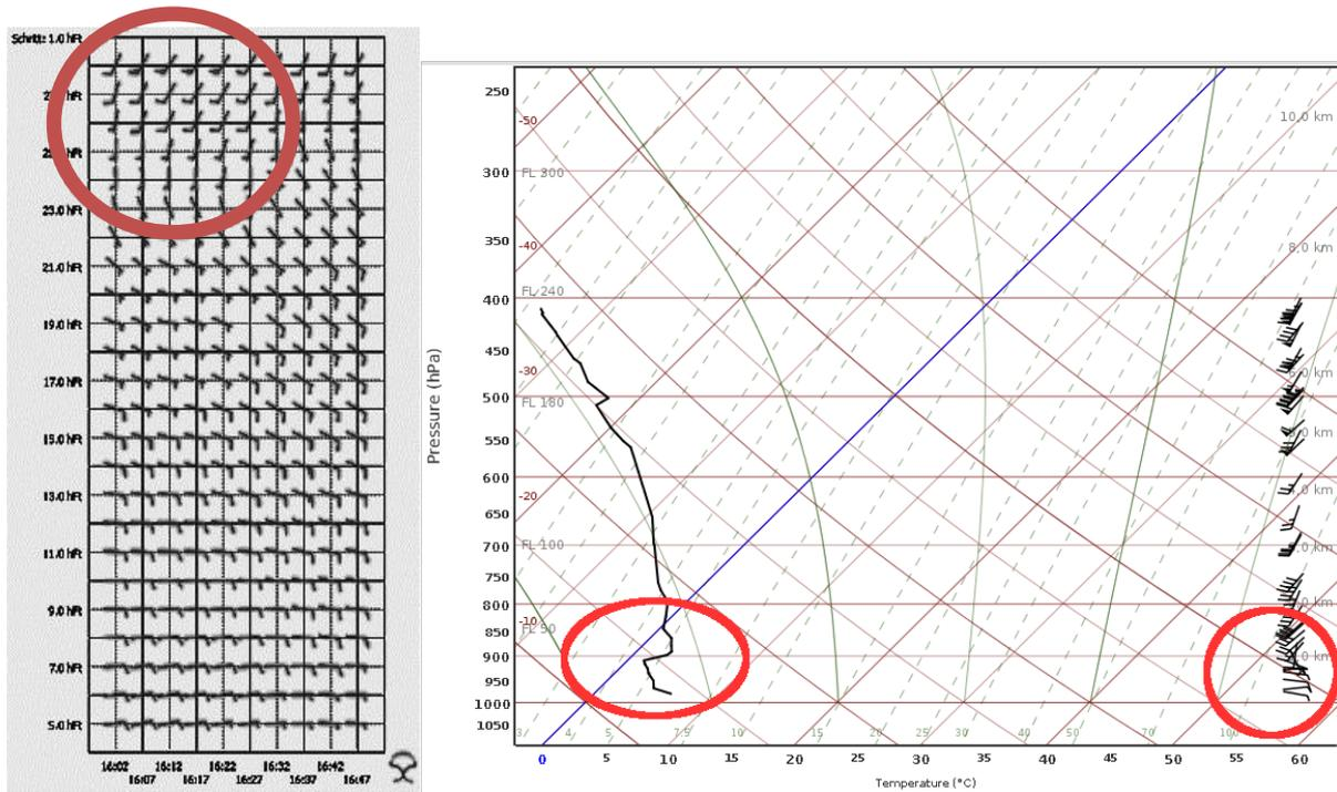
**Figure 10:** LLWAS VVP wind barb profiles (left panel) and AMDAR temperature and wind barb profile (right panel) at MUC. Date: 17 February 2014, 16:02 UTC till 16:47 UTC for LLWAS wind and about 16:45 UTC for AMDAR temperature and wind.
