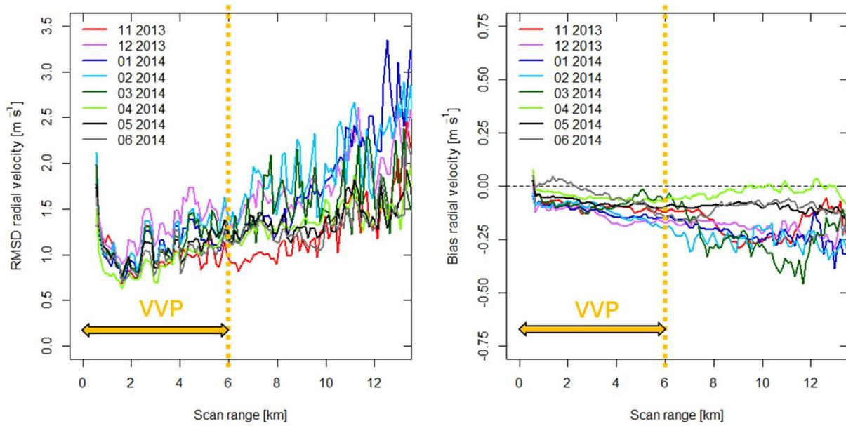
Figure 6: Mean monthly lidar–radar RMSD (left) and bias (right) of 3° PPI radial velocity for FRA; as function of range.
