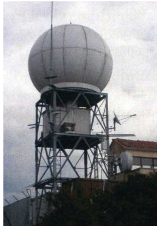
Fig. 3. The antenna of the C-Band radar.
