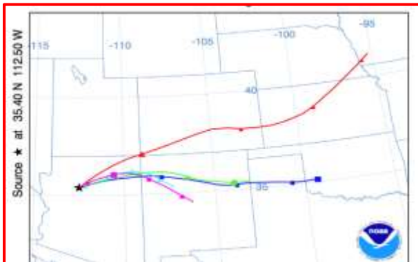
Fig. 16. Particle trajectory estimated using the NOAA Hysplit model for the flight period on 26 March 2014.
