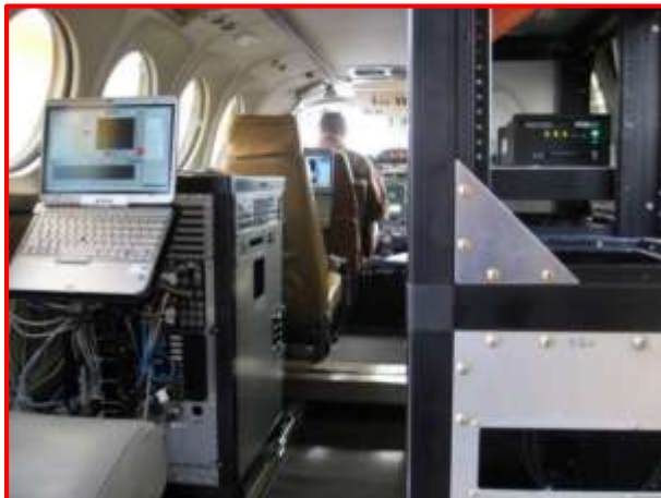
Fig. 5. Interior view of UW King Air from entryway, showing instrument racks and data visualization computers used by the UW lead scientist and Embry-Riddle participants.
