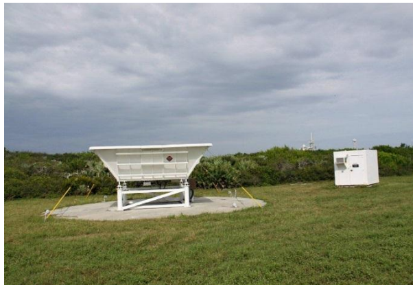
Figure 3: Picture of a 915-MHz DRWP at the ER (bottom, 45 th Space Wing 2013).
