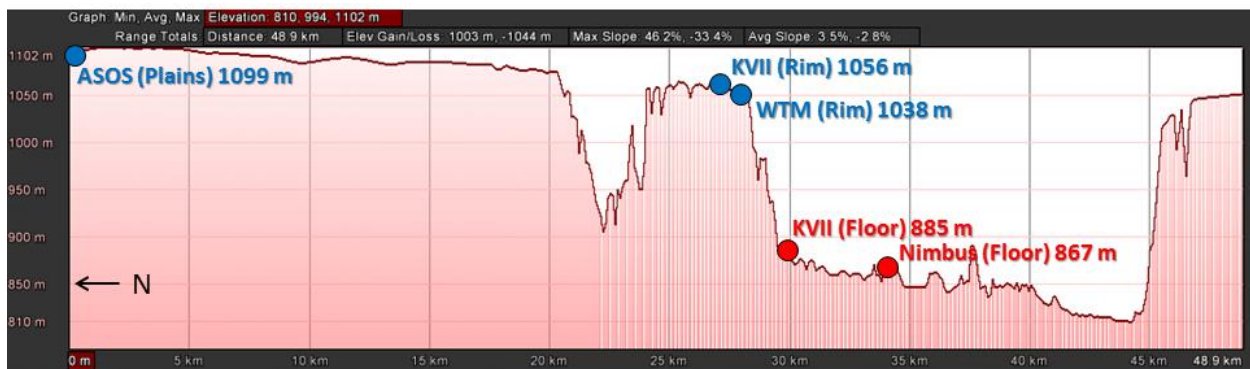
Figure 4: Topographical cross-section of Palo Duro Canyon with the location and elevation of meteorological instruments utilized in this study noted.
