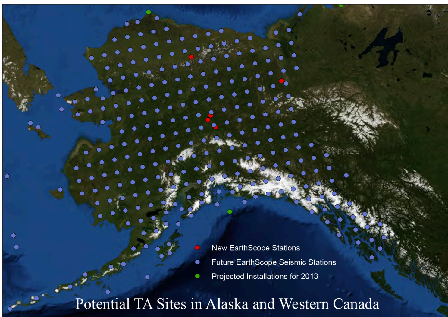
Figure 1 – Original hypothesized deployment for the USArray TA footprint throughout Alaska and into Canada from 2012. Red circles represent sites that already were installed at this time in 2012, blue circles indicate potential sites, and green circles represent sites that were already surveyed and at the time were planned for installation. The main purpose of this figure is to indicate that the objective of the Alaskan deployment is the same as in the Lower 48: to provide a Cartesian grid deployment of seismic stations at a ~85 km grid space interval for the purpose of monitoring the interior of the Earth.
