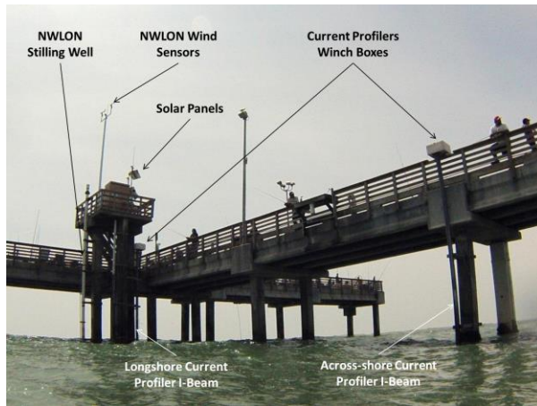
Figure 2. Illustration of the overall experimental geometry with the locations of both the offshore and the nearshore looking current profilers at the seaward end of Bob Hall pier.
