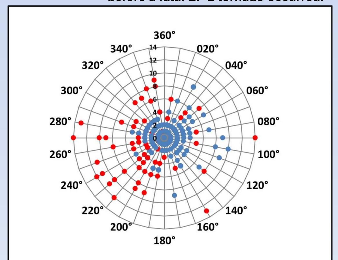
This polar plot represents the relative positions of K<sub>DP</sub> maxima (red dots for tornadic cases and blue dots for non-tornadic) versus Z<sub>DR</sub> maxima (the center point).
