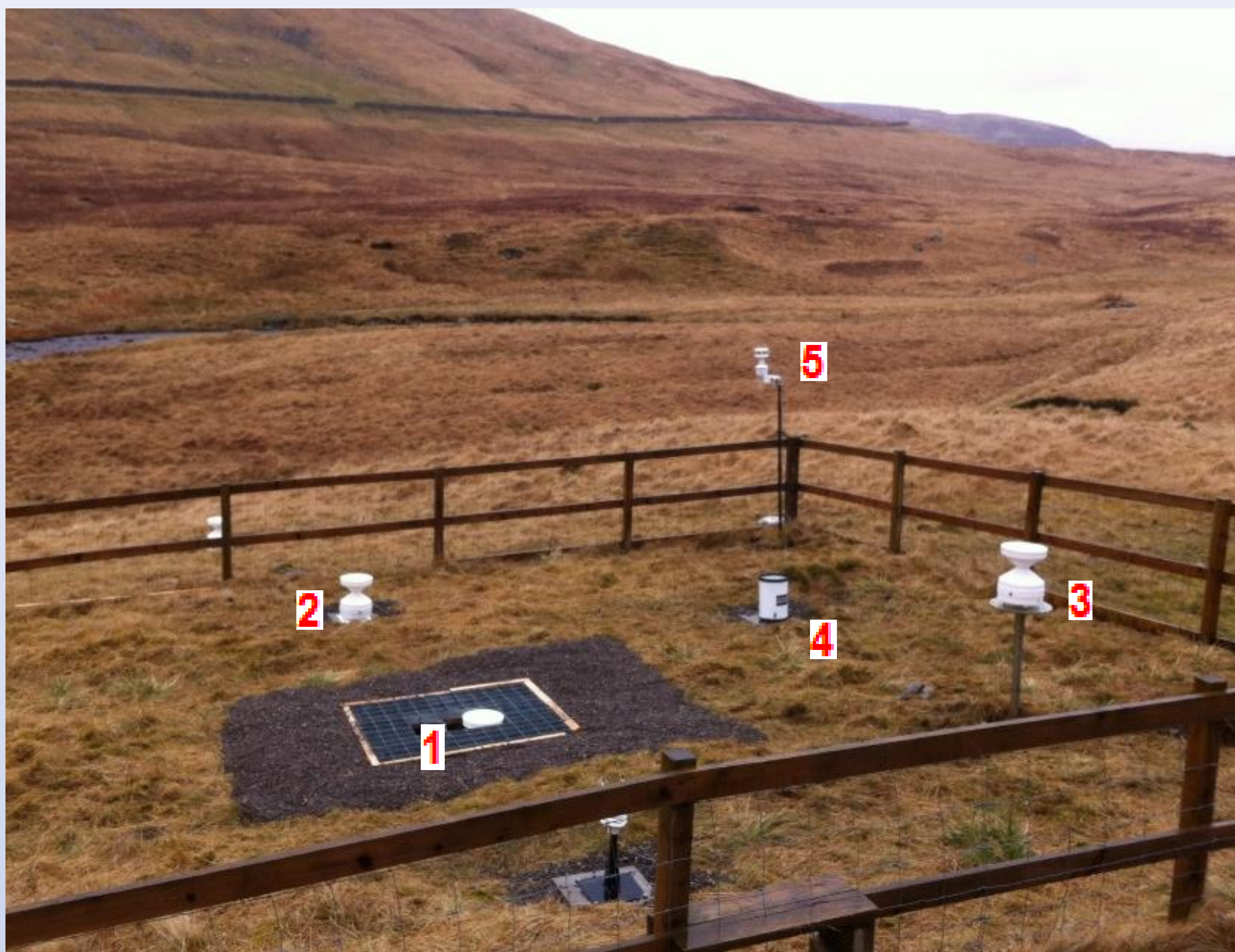
Figure 1. Talla Water research station, Scottish Borders. Elevation: 430m. Identical aerodynamic rain gauges (ARG100s) are mounted at different heights: reference pit gauge (1), ground-mounted gauge (2), 1-metre mounted gauge (3). There is also a ground mounted straight-sided gauge (4) and wind speed measurement at two metres (5). This upland site is situated at the top of a valley running east-west, with strong winds observed. (Picture by M.Pollock, April 2015. With thanks to University of Dundee/British Geological Survey/Borders Forest Trust for site provision).
