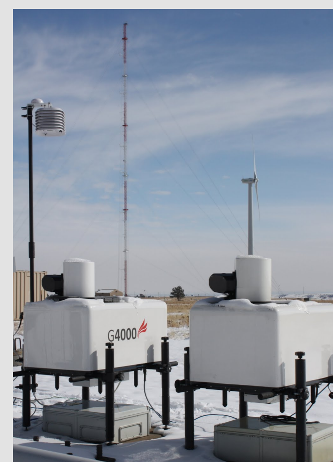
Figure 1. Galion lidars deployed near met tower at the National Wind Technology Center. Photo by Andrew Clifton, NREL 24390
