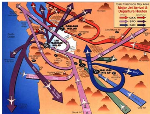
Figure 2: The Flight Paths of the Bay Area Airports including SFO. SFO's Bridge Approach which contains the stratus problem is in the light purple.
