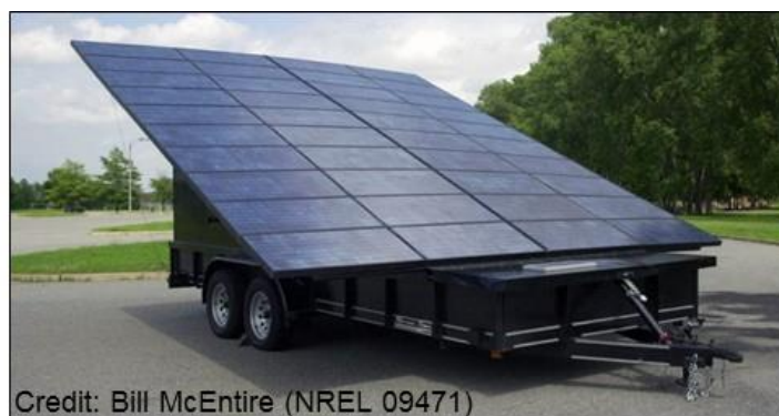
Fig. 2 A portable solar generator with battery storage (Morley 2015; Crow 2015)
