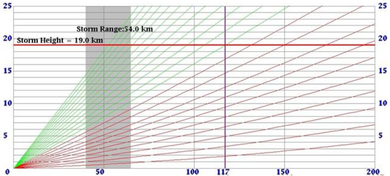
Fig. 3: Volume coverage pattern (VCP) generated by the range-based VCP algorithm for storm 3 at 153507 CDT. Red lines represent split cut (two PRTs) and green uniform (single PRT) waveforms.
