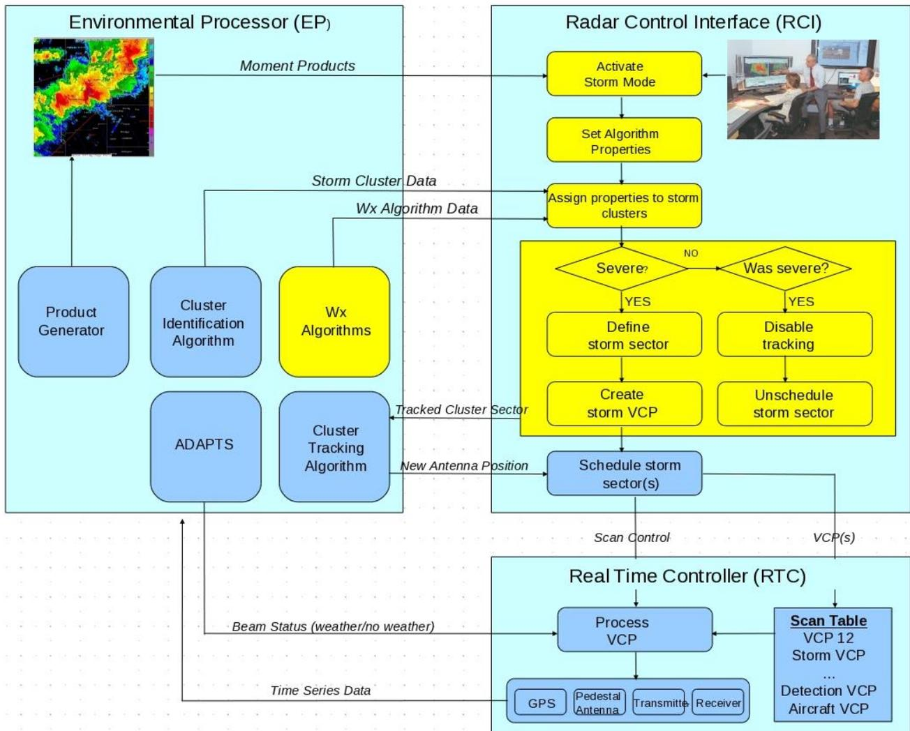
Fig. 1: Functional diagram of the adaptive scanning process at the NWRT PAR. Yellow regions highlight areas involved in the algorithm controlled part of the process.
