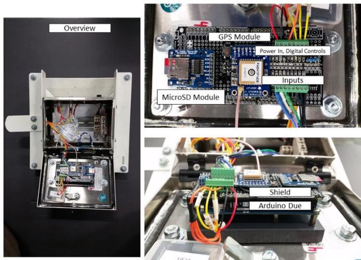
Figure 2. Photograph of the integrated Arduino Due and shield containing a microSD and GPS modules.
