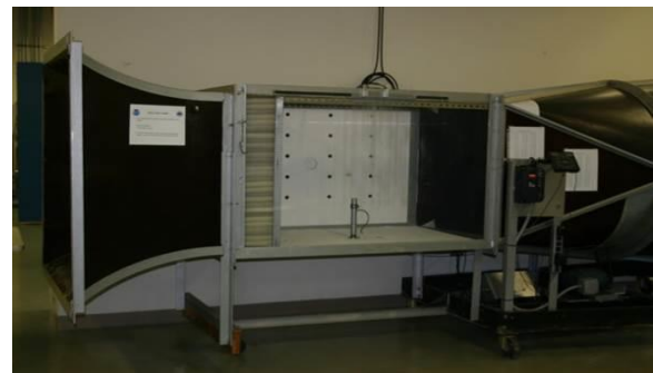
Figure 2. Low Speed Wind tunnel. 3'x3' section shown.
