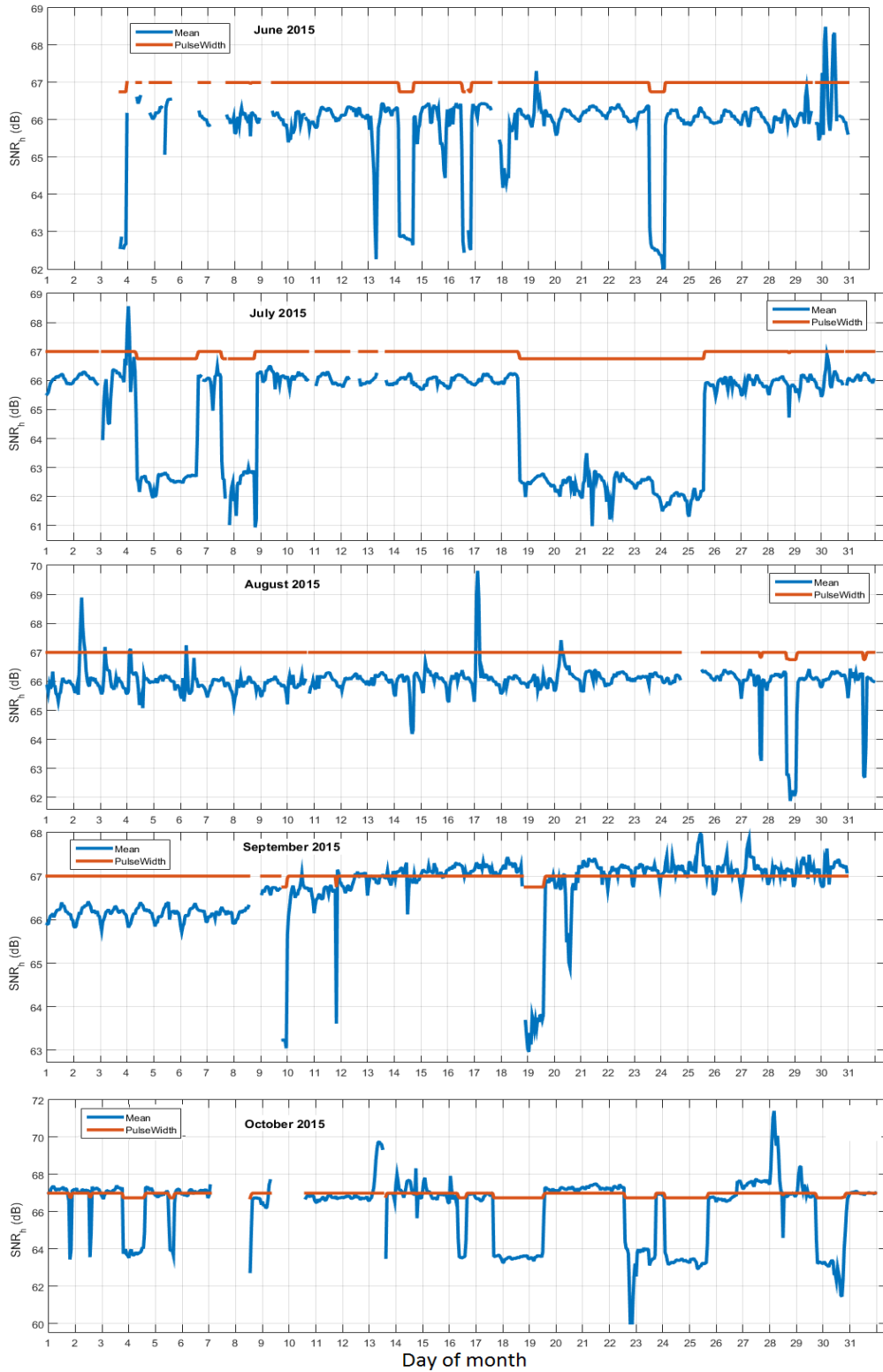
Fig. 5. Mean SNR h from ground clutter (the blue line) from June to October 2015. WSR-88D KOUN. The brown line represents the pulse width. The higher line corresponds to the long radar pulse and the lower one represents the short pulse.
