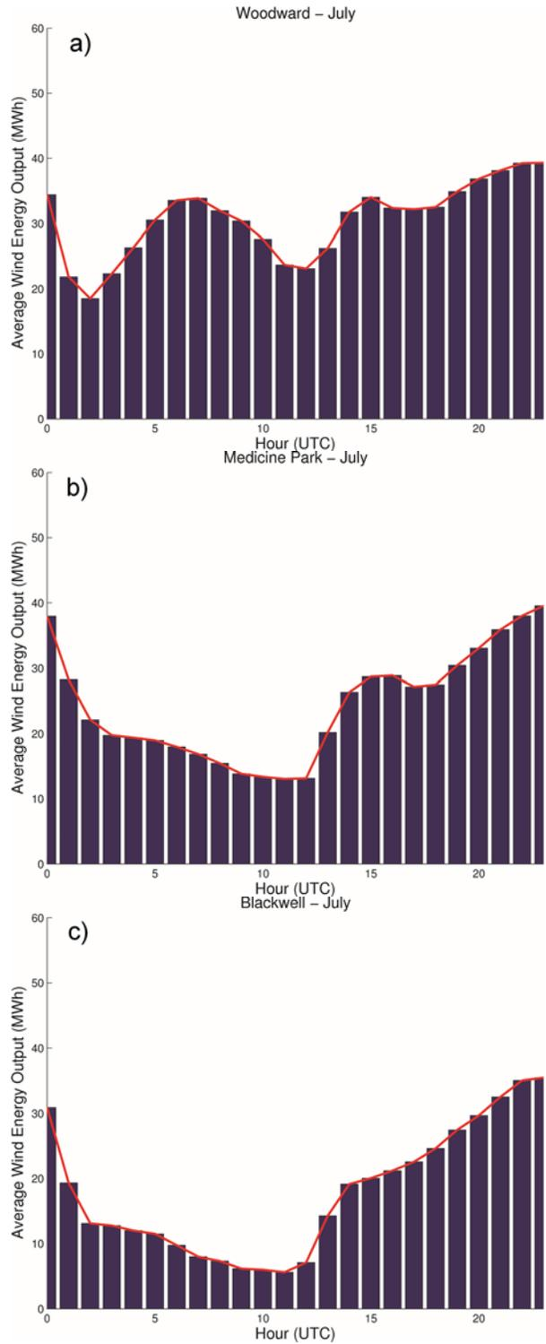
Figure 4 Average wind energy output (MWh) for each hour (UTC) during the month of July, for a) Woodward, b) Medicine Park, c) Blackwell, Oklahoma for a 100 MW rated system over the period 1996-2015.
