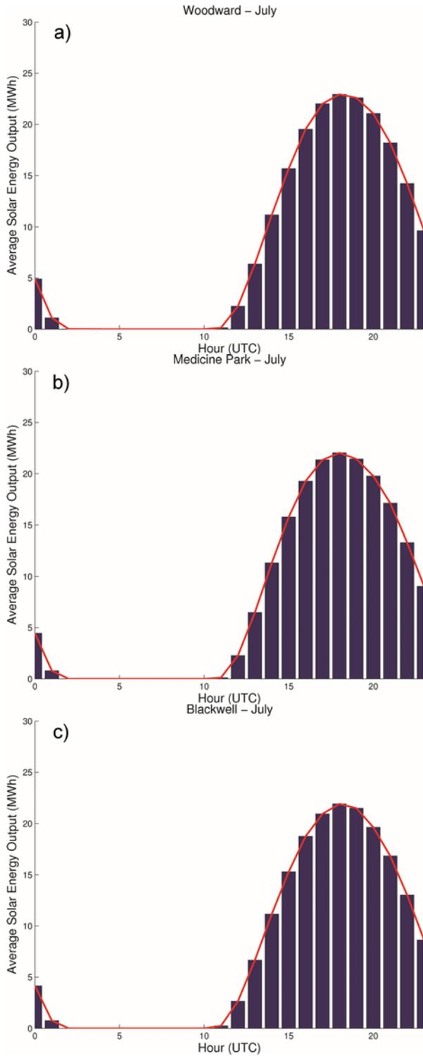
Figure 3 Average solar energy output (MWh) for each hour (UTC) during the month of July, for a) Woodward, b) Medicine Park, c) Blackwell, Oklahoma for a 30 MW rated system (with fixed tilt of 35°) over the period 1996-2015.
