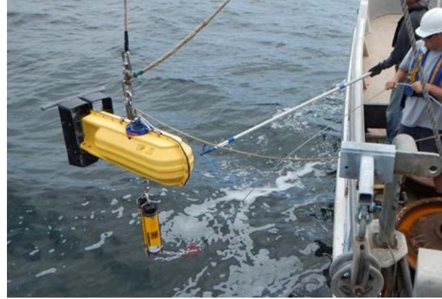
Figure 2. An example of one type of bottom mounted platform (left) and subsurface buoy mount (right) used for deployments.
