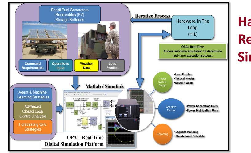
Hardware in the Loop Real Time Digital Simulation
