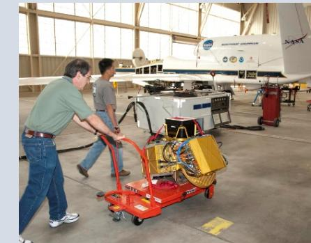
Dual-frequency conical scanning radar
