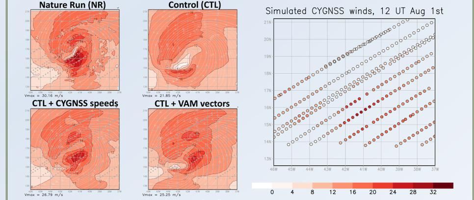
Fig 5. Layer-average, near-surface wind speed and streamlines [lowest 30 mb] from the Nature Run (NR) and from the analysis of three OSSEs, valid at 1200 UT August 1. The storm is just forming in all DA treatments, as in the NR, but with a significant southwest displacement compared to the NR. Wind speed is shaded according to the color scale in Fig. 6.
