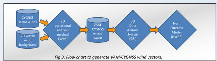
Fig 3. Flow chart to generate VAM-CYGNSS wind vectors.
