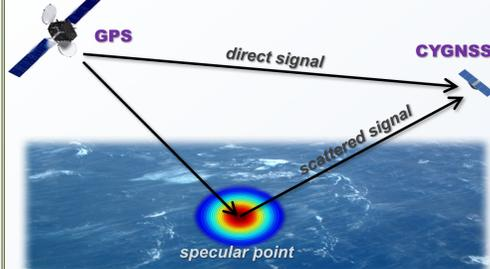
Fig 1. Geometry of GPS-based quasi-specular surface scattering. The GPS direct signal provides location, timing, and frequency references, while the forward scattered signal contains ocean surface information.
