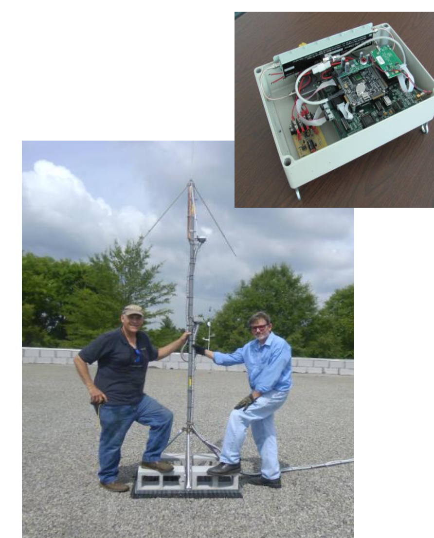
Figure 5: LMA sensor box and a typical antenna installation
